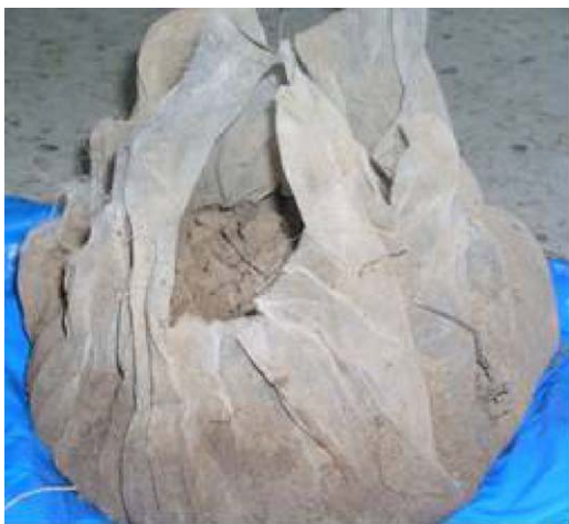
Figure 2. Typical PP net-pouch with 3 kg soil from the experimental field containing an LLDPE-P1 film sample. [Color figure can be viewed in the online issue, which is available at wileyonlinelibrary.com .]
